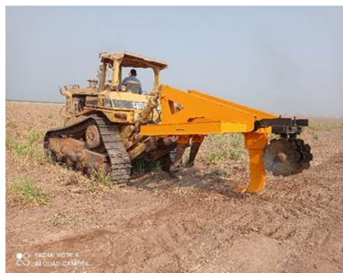
Figure 1. Combined two-level deep tillage machine cum with a conical-type disc gang.
