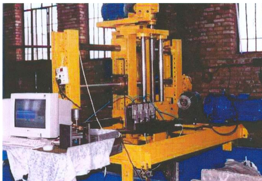
Figure 7. The test rig connected to one of the four force magnifying cylinders and its load cell to test their performance.
