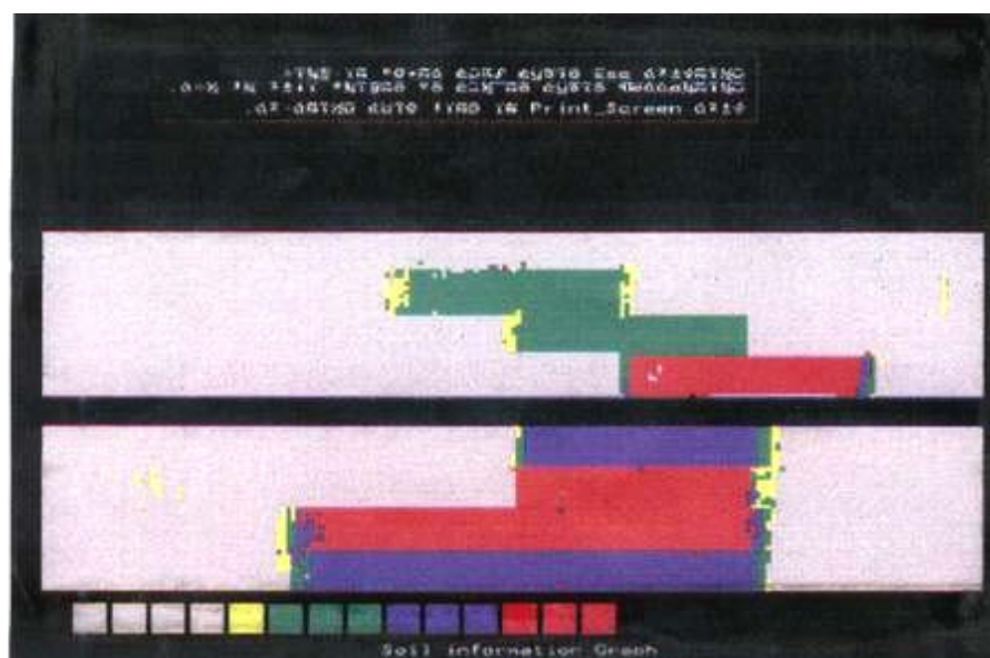
Figure 15. Soil compaction map of the hard pan configuration arranged in the soil bin as shown in Figure 8.
