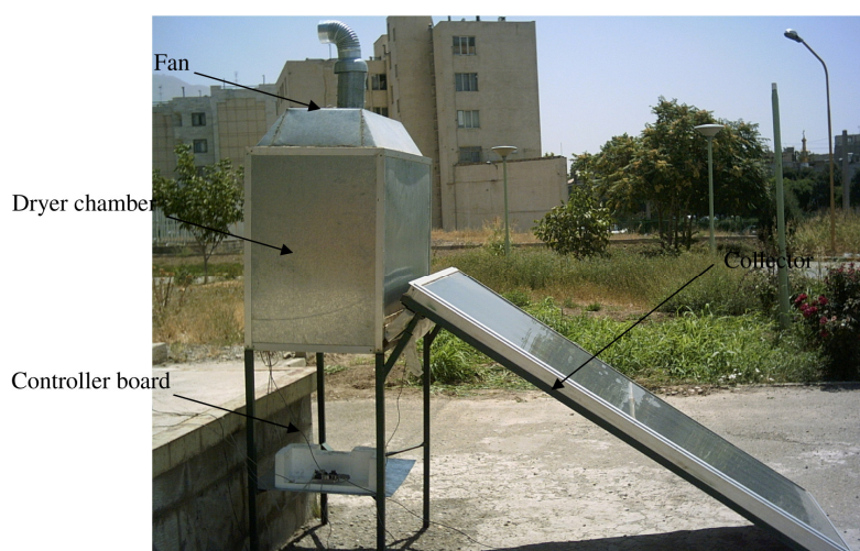
Figure 1. Experimental forced convection solar dryer.
