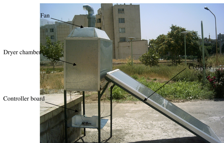
Figure 1. Experimental forced convection solar dryer.
