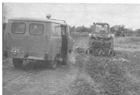
Figure 2. Determination of the energetic and ergonomic parameters of the designed transplanter using a mobile laboratory.
