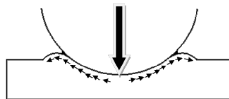
Figure 9. The schematic longitudinal view of how gelatin materials of Aloe vera shift the pressure range to the lower surface of the upper rind
