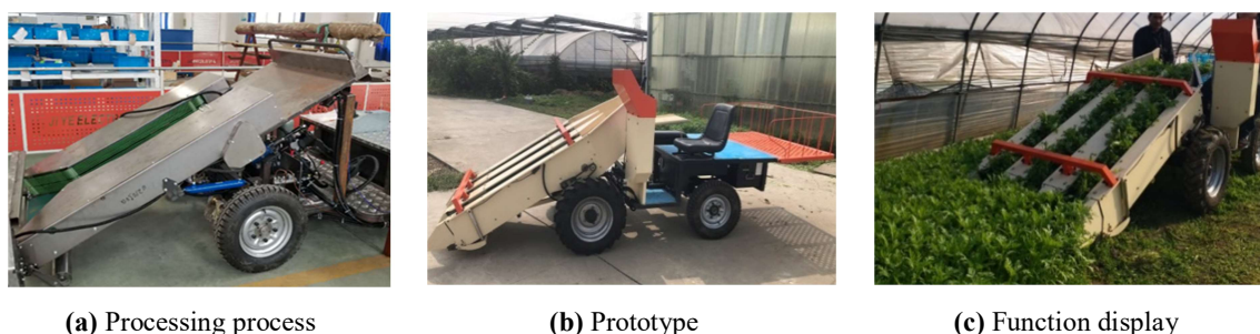
Figure 12. Prototype of self-propelled intelligent small green vegetables combine harvester.
