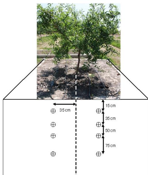
**Figure 1.** Drainage lysimeter used for the experiment with TDR probe distribution across the soil profile.
