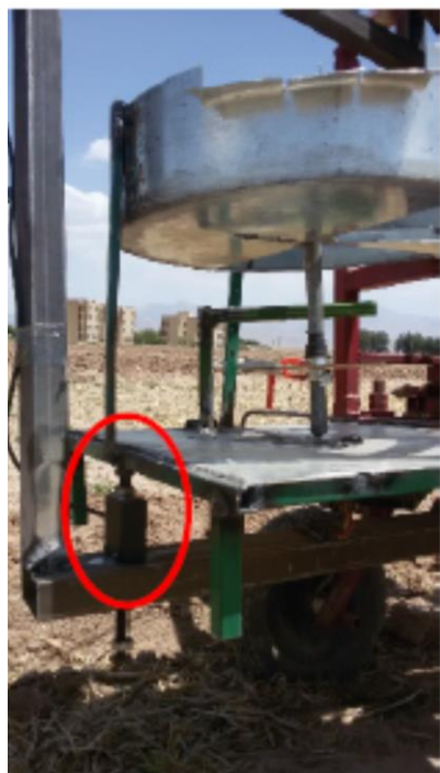
Figure 5. Load cell installation on prototype under YMS.
