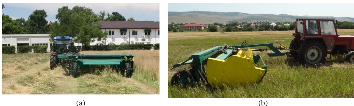
Figure 3. The trailed vindrover on experimental plots: (a) INMA Bucharest field, (b) SCDP Vaslui field.
