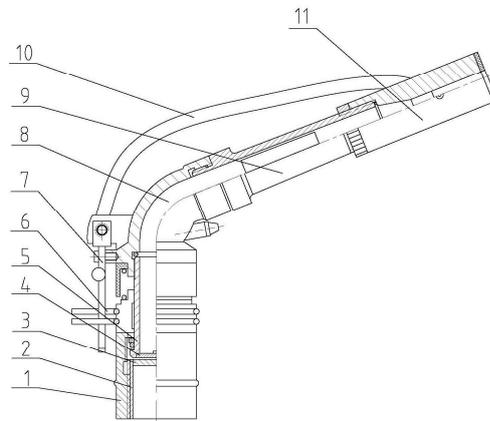
**Figure 2.** The structure of the new fluidic sprinkler with a pressure-adjusting device. (1) Swivel connection; (2) Connecting sleeve; (3) Static insert; (4) Movement insert; (5) Hollow shaft; (6) Location limit device; (7) Reversing device; (8) Spraying body; (9) Spraying pipe; (10) Plastic tube, (11) Nozzle.
