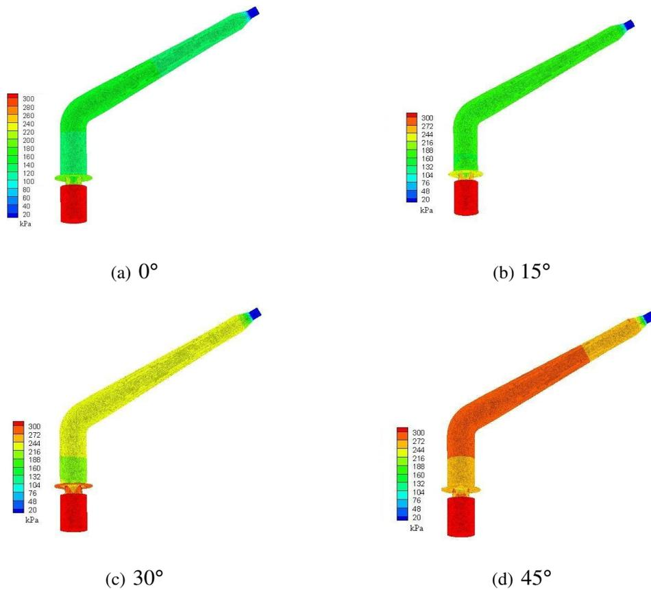
Figure 12. The pressure distribution of the sprinkler.
