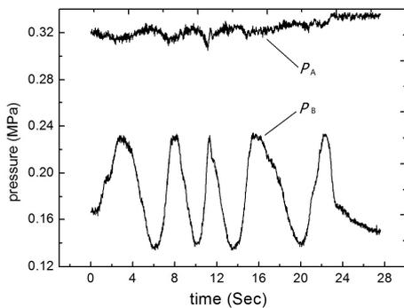
Figure 14. Pressure values for sections A and B.
