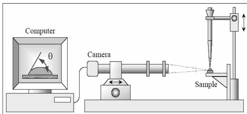
Figure 1. Scheme of contact angle determination device.
