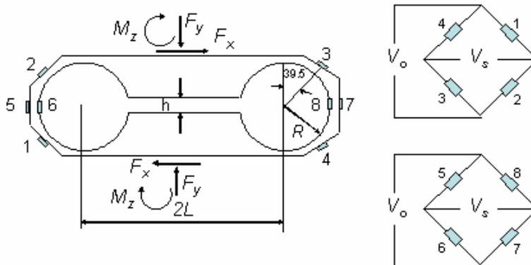
**Figure 6.** Stress nodes and strain gage locations in the extended octagonal ring. Bridge containing gages 1, 2, 3, and 4 is sensitive to  $F_x$  while the bridge containing gages 5, 6, 7, and 8 is sensitive to  $F_y$ .
