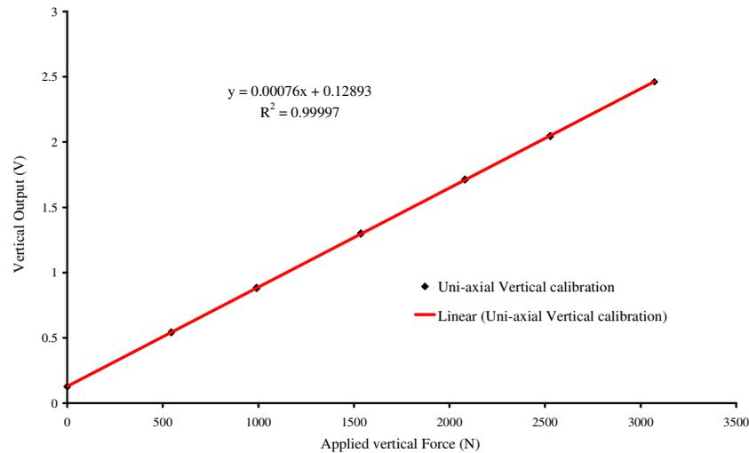
**Figure 9.** Evaluation of vertical primary sensitivity of sensor
