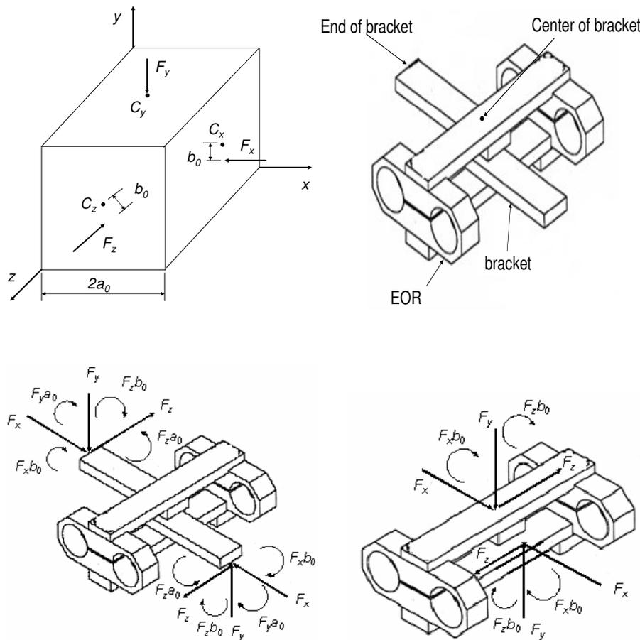
**Figure 1.** Forces transferred from covering plates to the extended octagonal ring (EORs): (a) Forces applied to the cover plates of the sensor; (b) Schematic of the sensor without cover plates; (c) Forces transferred from the covers to the hitch point of sensor, and (d) Forces transferred from the hitch point to the center of braces.
