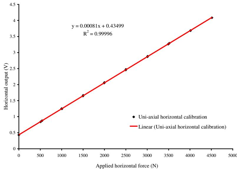
**Figure 8.** Evaluation of horizontal primary sensitivity of sensor.
