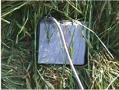
**Figure 12.** extended octagonal ring sensor placed inside the bale.
