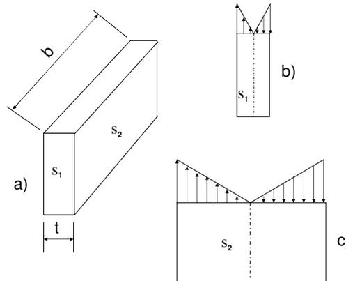
**Figure 4.** Bending stresses applied to the ring section of the sensor: (a) A section of the flexible part (ring section) of the sensor; (b) Bending stress applied by  $F_x$  and  $F_y$  on the cross-section of the ring, and (c) Bending stress applied by  $F_z$  on the cross-section of the ring .
