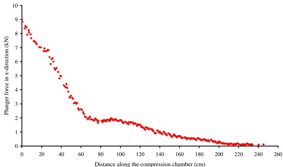
**Figure 14.** Plunger forces recorded by the designed transducer in the x-direction inside the bale chamber of a large square baler for baling barley straw.
