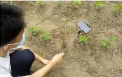
Figure 2. Acquiring canopy image using a smartphone camera fixed with the selfie stick under natural light in field (online color).
