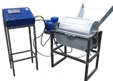
Figure 8. Forage chopper after final assembly.
