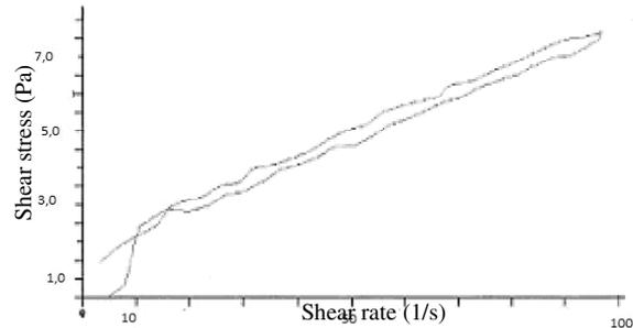
**Figure 2.** Thixogram of the hydrogel chitosan 0.5% at 25°C.
