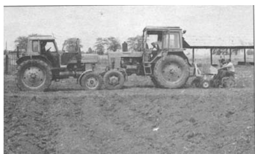
Figure 3. Method of determining required draft.
