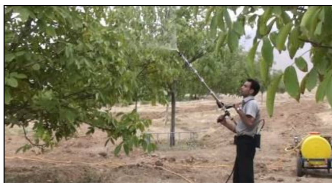
Figure 5. Designed and fabricated telescopic sprayer in operation.
