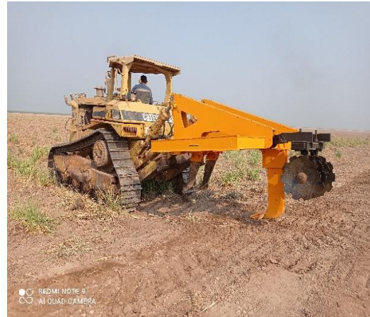
119 Fig. 1. Combined two-level deep tillage machine cum with a conical-type disc gang.
