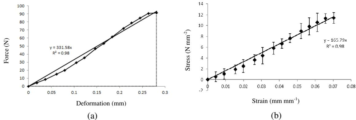
**Figure 3.** A typical force-deformation curve of wheat grain: (a) Fitted line and the approximate triangular shaped area for calculating static toughness, and (b) Fitted line through the stress-strain data point for calculating the apparent elastic modulus.
