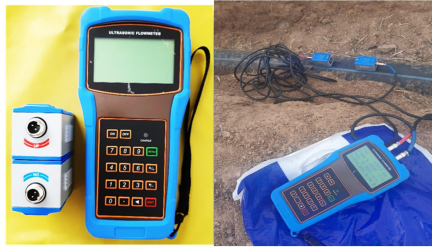
Figure 2. Portable ultrasonic flow meter was used in this study.
