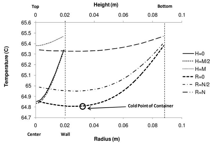
**Figure 5.** Evolution of predicted temperatures at three radii (center, middle and wall) along the vertical axis and at three heights (bottom, middle and top) along the radial axis of the jar after 3,000 seconds heating at 65°C. (Dashed lines are representing wall and bottom of container, respectively).
