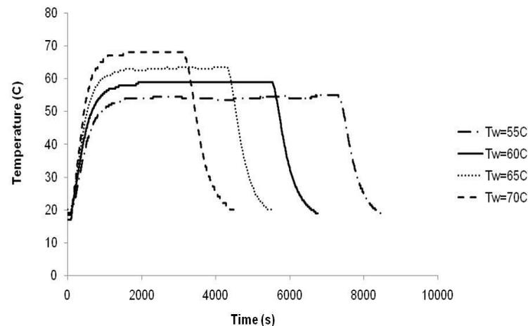
**Figure 2.** Experimental heat penetration curves in caviar jar during pasteurization in water bath (Experimental values were measured in the caviar geometric center).
