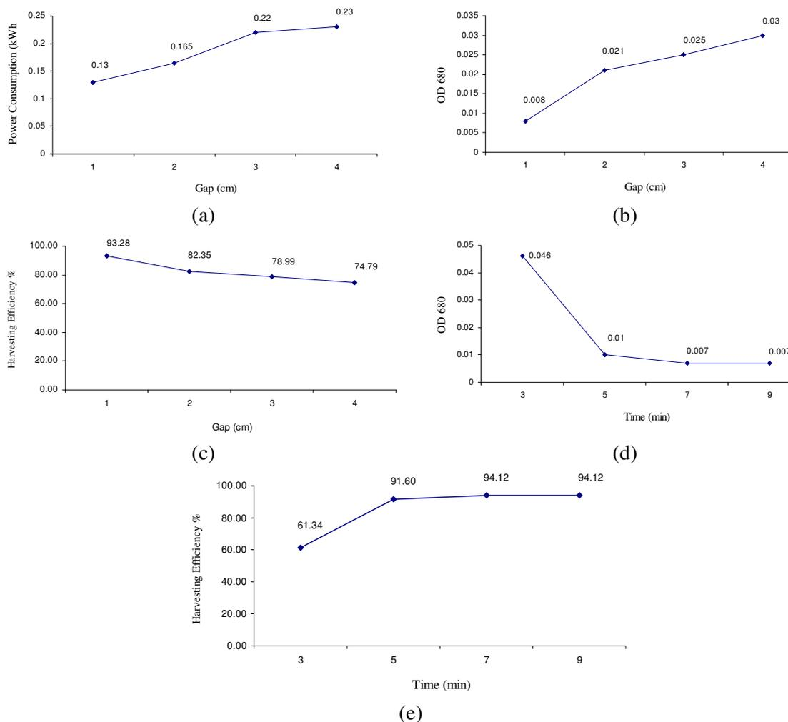
**Figure 6.** Effect of (a) electrode gap on energy consumption (b) electrode gap on optical density after electroflocculation (c) electrode gap on harvesting efficiency (d) electroflocculation time on optical density (e) electroflocculation time on harvesting efficiency, at fixed current density of  $50 \text{ A m}^{-2}$ , and a solution with  $EC = 1.35 \text{ S m}^{-1}$ .
