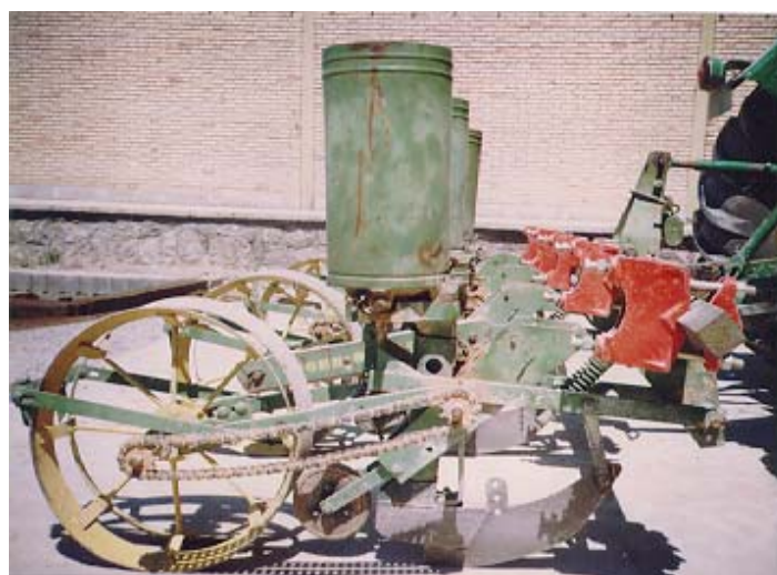
Figure 2. John Deere cotton planter with open center concave steel press wheels.
