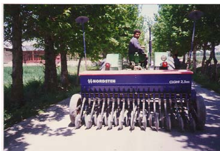
Figure 3. Nordsten grain drill with single disk openers.
