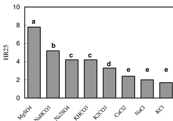
**Figure 4.** Comparison of the mean hydrometer readings of pure solution of different salt types corrected for 25 °C. The small letters on the bars are the rankings based on Duncan's Multiple Range Test (p=0.01).
