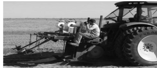
Figure 1. SWRT membrane installation equipment (Smucker and Basso, 2014).
