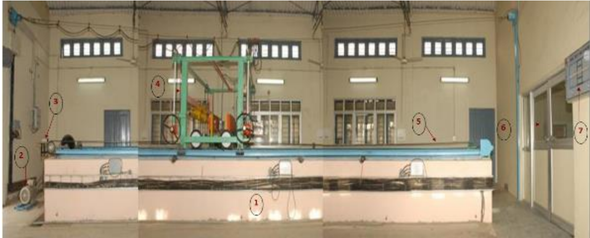
Figure 1. A view of soil bin system: 1. Rectangular soil bin; 2. Variable speed motor; 3. Linear speed sensor; 4. Tool and instrumentation carriage; 5. Chain drive and guide rail; 6. Control room, 7. Mimic panel.
