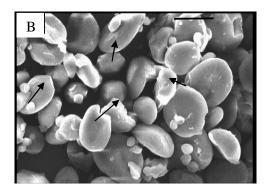
**Figure 1**. Scanning electron micrographs of the cross-linked wheat starch before (A) and after (B) treatment with L-ascorbic acid. Each bar on the micrographs is 20 μm.
