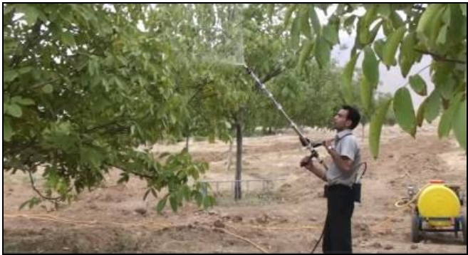
Figure 5. Designed and fabricated telescoping sprayer in operation.
