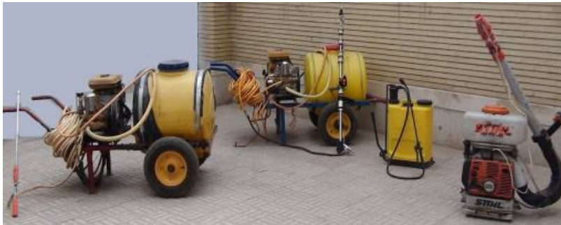
Figure 6. Sprayers used in the study (From right to left: Atomizer equipped with electrostatic head, side pump, wheel barrow equipped with telescoping boom, wheel barrow with normal lance).
