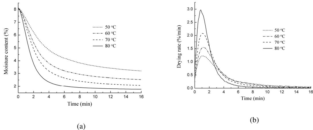
**Figure 1.** Drying curves of wheat straw (a) Drying rate curves of wheat straw (b) at different temperatures.
