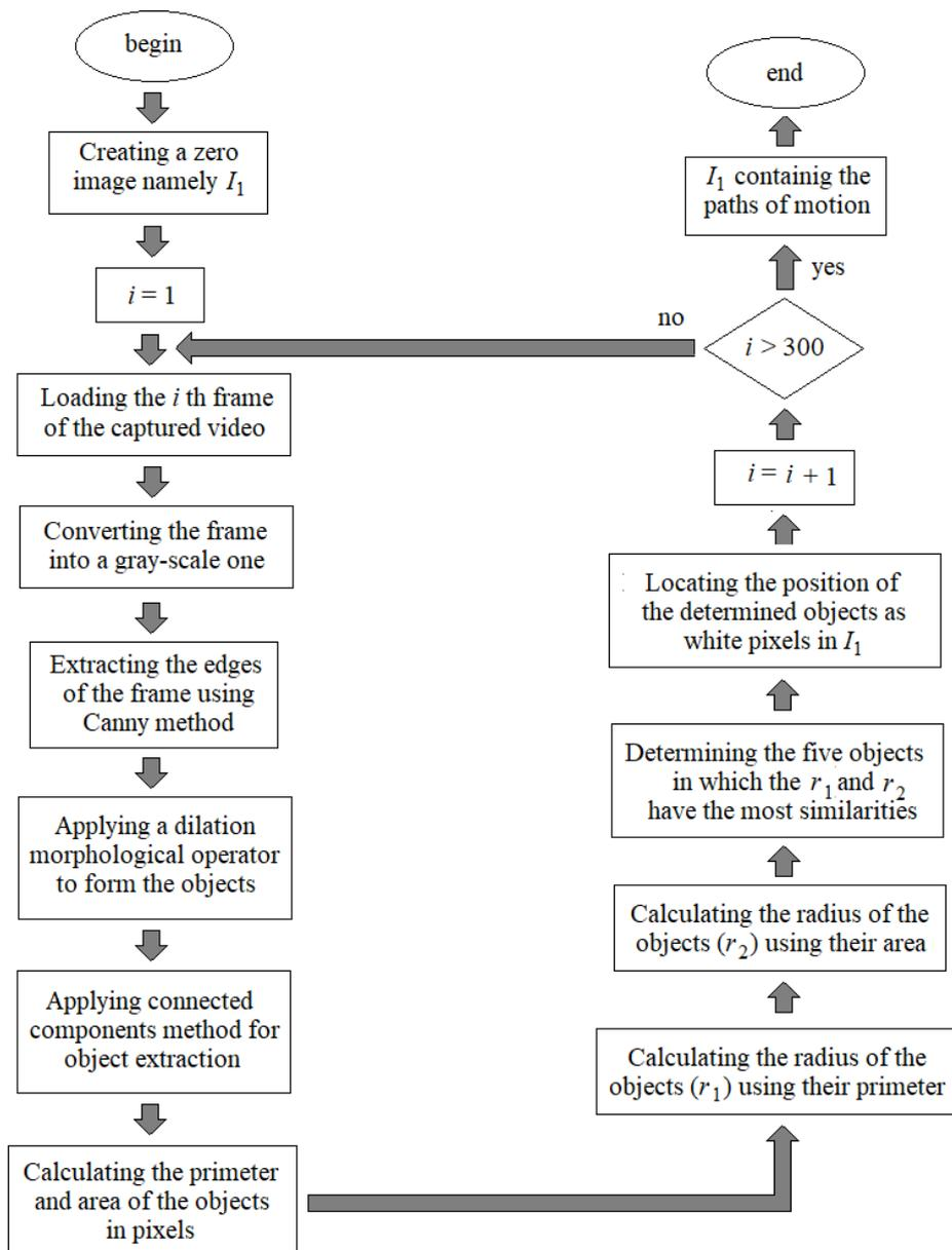
**Figure 5.** The flow chart of the image processing algorithm used for tracking the motion of the pins.
