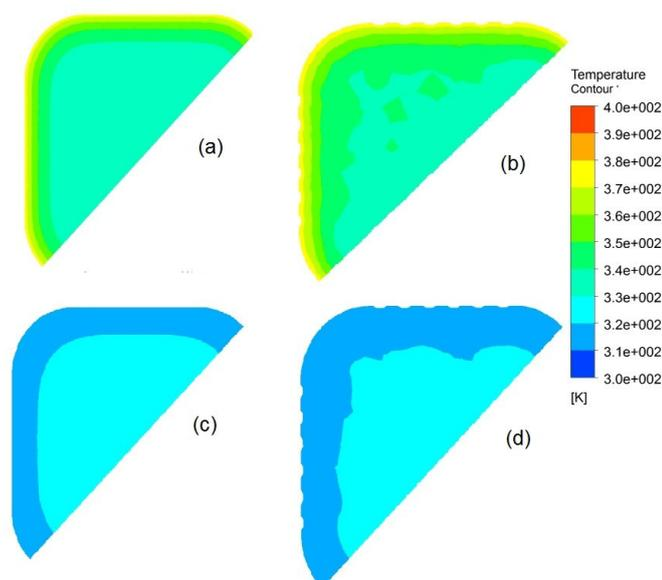
**Figure 5.** Temperature distribution in  $Z=13.75$  mm (a, b): At 3,600 seconds for straight wall container and wrinkled wall container, respectively, and (c, d): At 48,000 seconds for straight wall container and wrinkled wall container, respectively.
