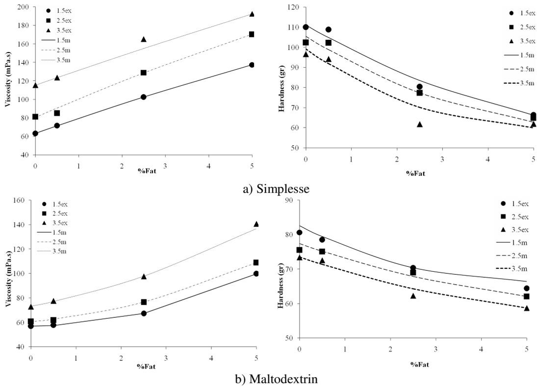
**Figure 3.** A comparison of the experimental and the predictive functional properties (viscosity and hardness) obtained by the model as a function of fat content and at different fat replacer contents.
