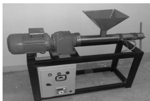
Figure 11. Side view of the oil extraction machine.
