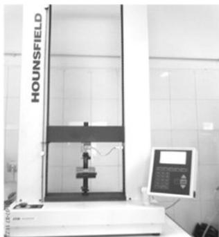
Figure 2. Materials testing machine
