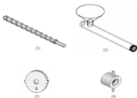
Figure 10. 1. Screw, 2. Barrel, 3. Die, 4. Cap.
