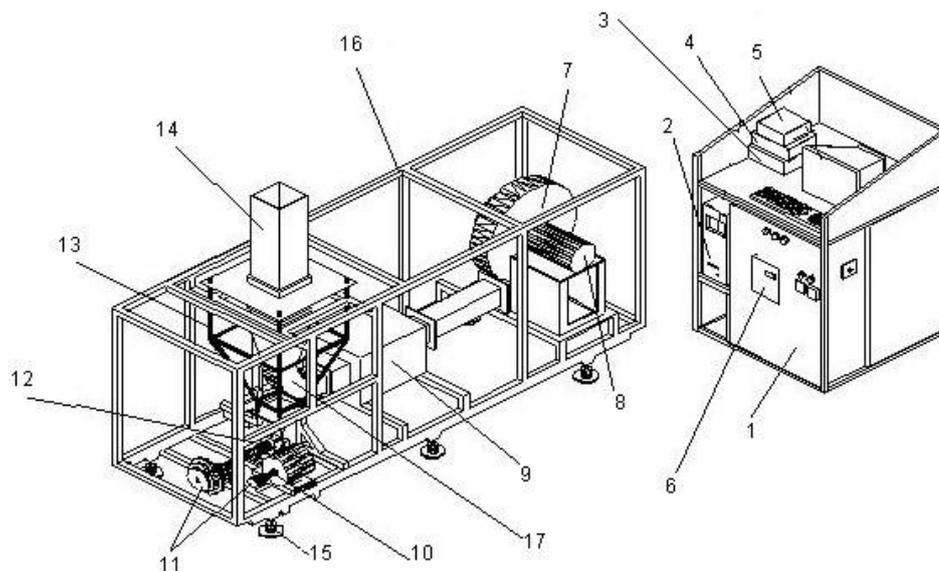
**Figure 1.** Schematic of experimental vibro-fluidized bed dryer: (1) Electrical unit; (2) Computer; (3) Power supply; (4) Main circuit and sensors amplifier circuit; (5) Relays circuit; (6) Inverter; (7) Blower; (8) Blower motor; (9) Electrical heater; (10) Vibration motor; (11) Pulleys; (12) Slider crank; (13) Vibratory arms; (14) Fluidization chamber; (15) Dampers; (16) Frame, (17) Elbow.
