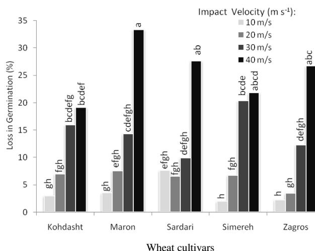
**Figure 3.** Effect of wheat cultivar and impact velocity interactions on the percentage of loss in germination of seeds.
