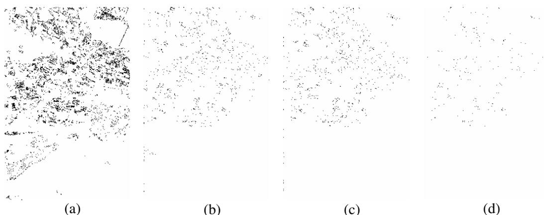
**Figure 3.** Alfalfa cover detection: (a) Pixels whose reflectance difference in bands 0.55  $\mu\text{m}$  and 0.67  $\mu\text{m}$  is 0.042; (b) Pixels whose reflectance difference in bands 1.06  $\mu\text{m}$  and 0.67  $\mu\text{m}$  is 0.557; (c) Pixels whose reflectance difference in bands 1.06 $\mu\text{m}$  and 0.55 $\mu\text{m}$  is 0.51, (d) Pixels having all conditions set in a, b and c.
