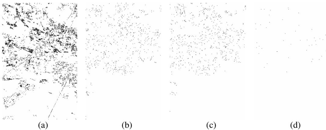
**Figure 5.** Wheat cover detection: (a) Pixels whose reflectance difference in bands 0.58  $\mu\text{m}$  and 0.64  $\mu\text{m}$  is 0.015; (b) Pixels whose reflectance difference in bands 1.080  $\mu\text{m}$  and 0.64  $\mu\text{m}$  is 0.459; (c) Pixels whose reflectance difference in bands 1.080  $\mu\text{m}$  and 0.40  $\mu\text{m}$  is 0.444, (d) Pixels having all conditions set in a, b and c.
