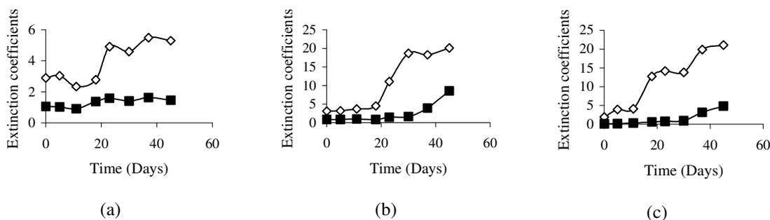
**Figure 2.** Change in specific extinctions at 232 nm (◇) and at 270 nm (■) during storage period at 65°C of raw sesame, sesame paste and olive oils. (a): Raw sesame oil; (b): Sesame paste oil, (c): Olive oil.
