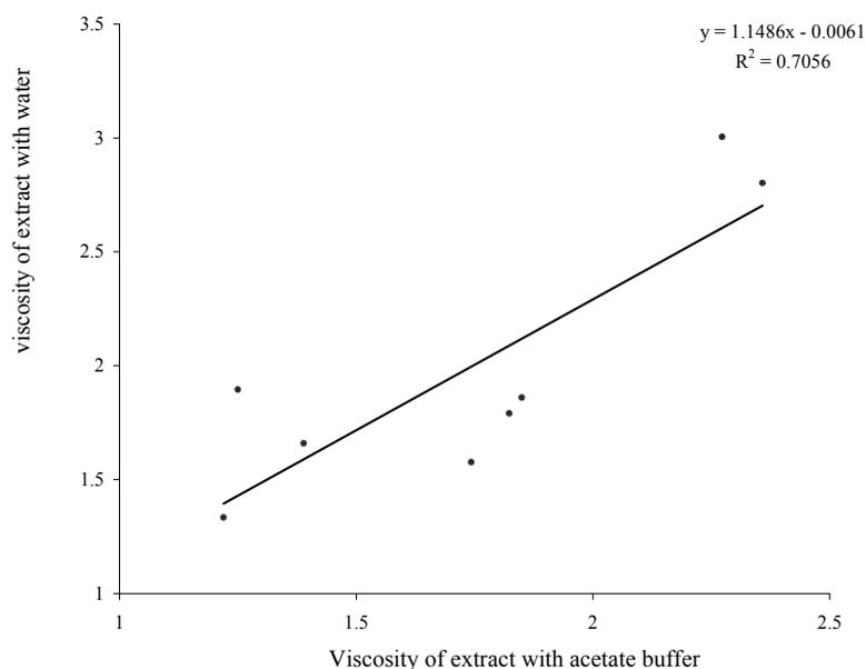
**Figure 1.** Correlation between two methods of viscosity measurement.
