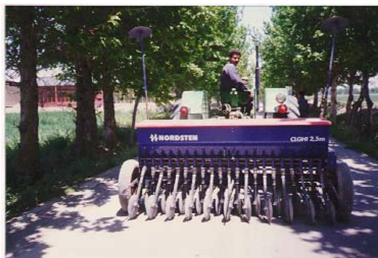
**Figure 3.** Nordsten grain drill with single disk openers.
