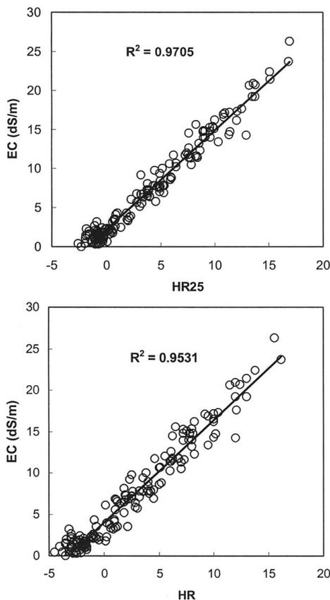
**Figure 2.** The relationship between the measured Electrical Conductivity (EC) and the Hydrometer readings corrected for 25°C (HR25) and uncorrected (HR) of the irrigation waters in Yazd Province, Iran.
