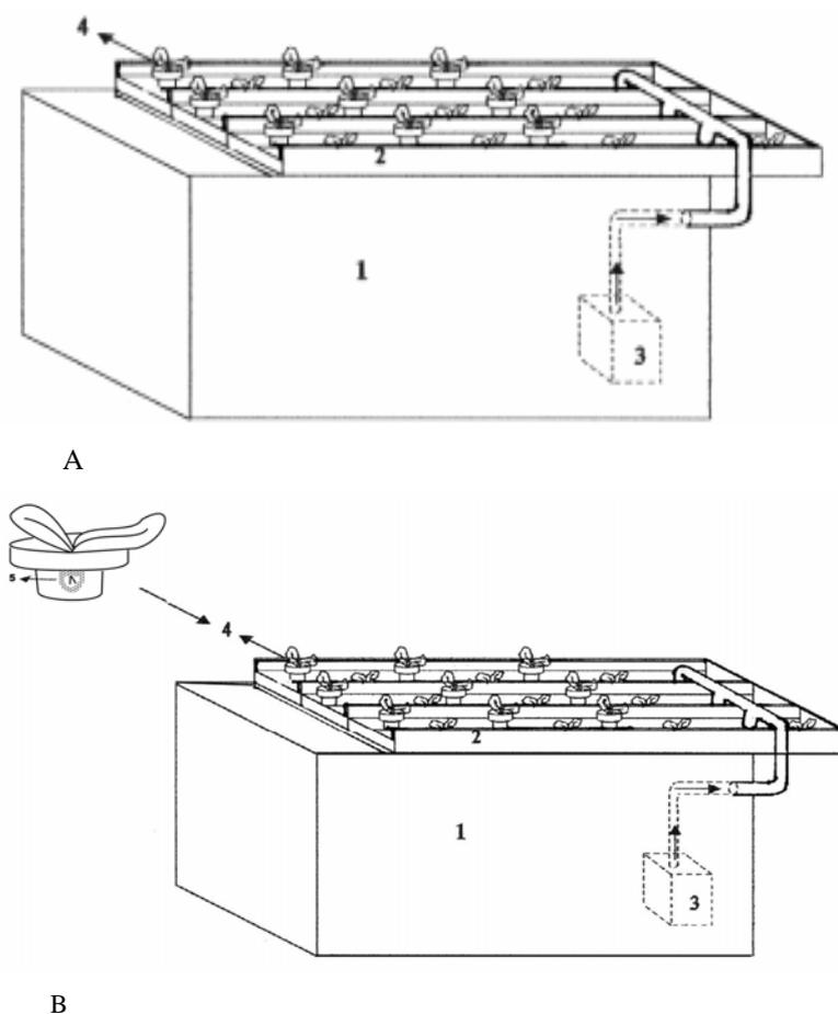
**Figure 1.** Schematic feature of the aquaponic system used for culture of fish and vegetables, 1. Fish tank, 2. Hydroponic troughs, 3. Water pump, 4. Lettuce cup, 5. A small cotton bag containing 10 g zeolite.
