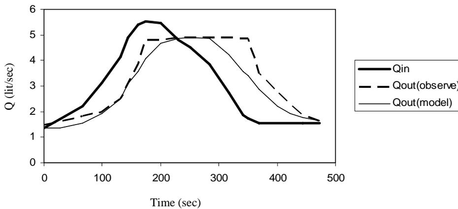
Figure 8. Three rockfill dams with an average particle size of 21 mm length of 0.5 m and distance between dams of 1.0 m. ( $R^2=91\%$ ).
