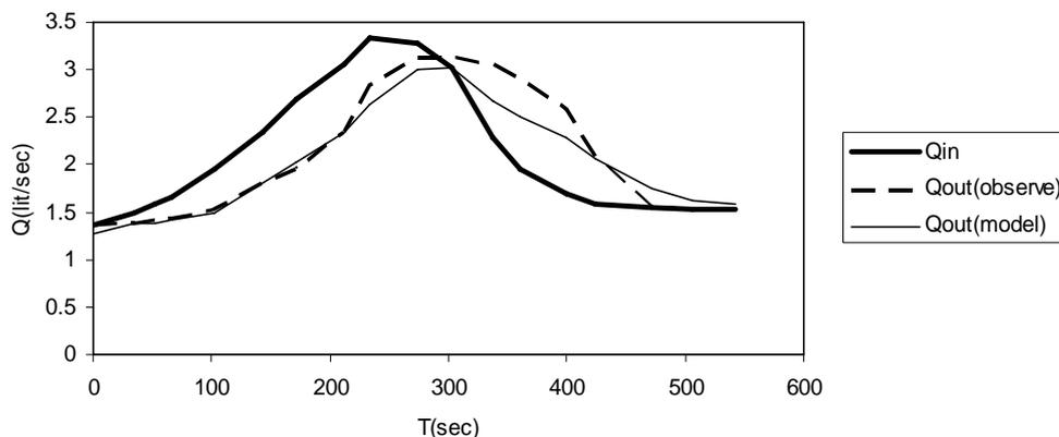
Figure 3. Two rockfill dams with a average particle size of 14.5 mm, length of 0.4 m and distance of 0.4 m ( $R^2=97\%$ ).
