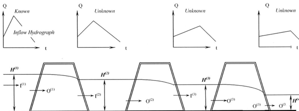
Figure 2. Routing through successive detention rockfill dams.
