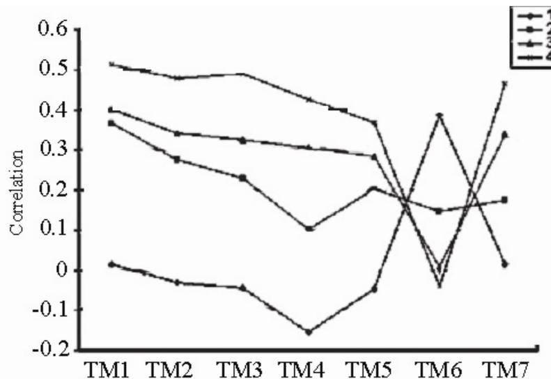
**Figure 6.** The plot of the correlation coefficients between the following soil salinity classes and DN values over TM bands of the Ardakan area: (1) Gypsiferous soils; (2) Total area (including non-saline, saline and gypsiferous soils); (3) Non-gypsiferous soil, (4) Non-gypsiferous soils with salinity conditions.
