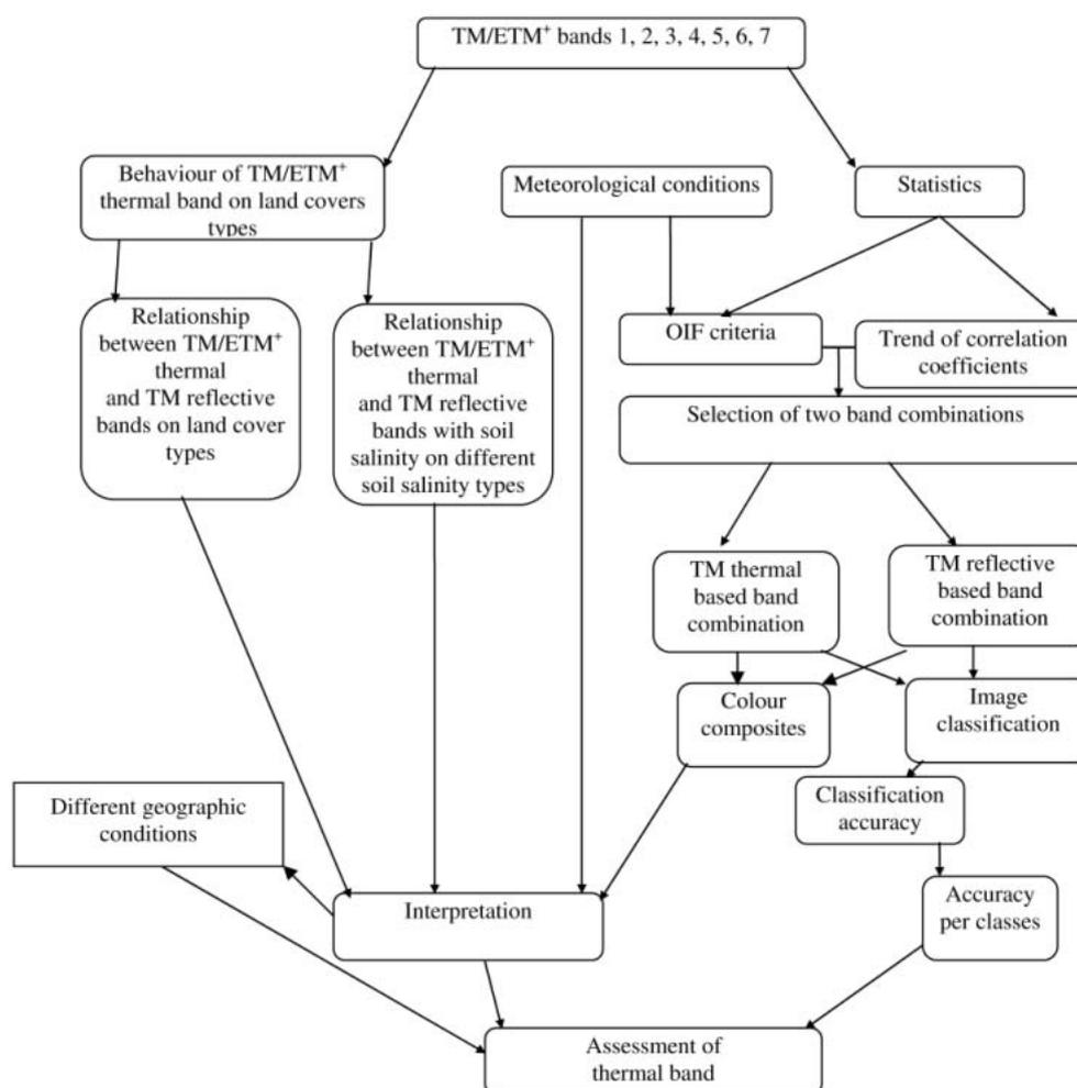
**Figure 2.** Flowchart of the proposed approach for evaluation of thermal band for soil salinity classification.
