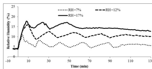
Figure 6. Variation of drying air RH at the flow rate of 0.012 kg s<sup>-1</sup>.
