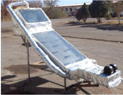
Figure 2. A photograph of the solar dryer equipped with the heat recovery system.
