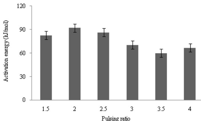
Figure 4. Activation energy under different levels of pulsing ratio.
