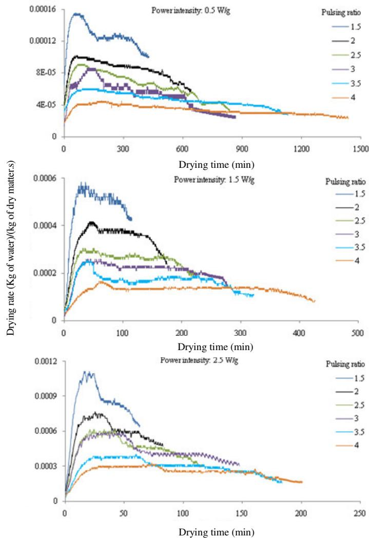
**Figure 2.** Variation of drying rate as a function of drying time at selected pulsing ratio and 0.5, 1.5 and 2.5 W g<sup>-1</sup> power intensities.
