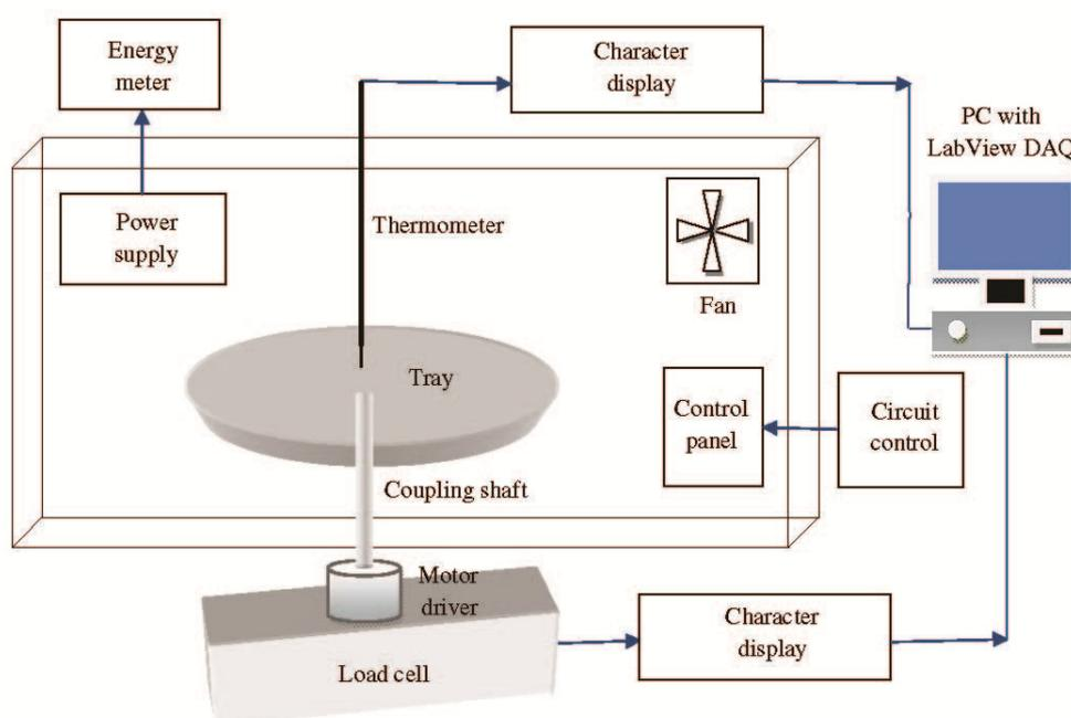
**Figure 1.** Schematic illustration of the MW drying system.
