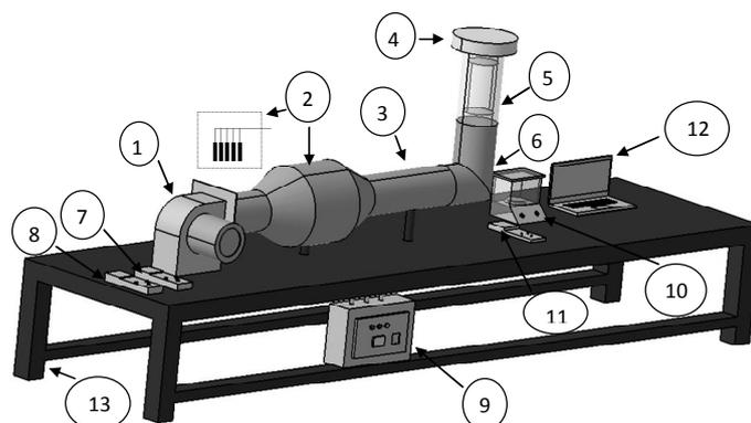
**Figure 1.** Schematic diagram of thin-layer dryer: (1) Fan and electrical motor; (2) Heating elements; (3) Duct and tunnel; (4) Chamber cap; (5) Drying chamber; (6) Mixing chamber; (7) Temperature and moisture meter; (8) Anemometer, (9) Thermostat and inverter; (10) Digital balance; (11) Input and output air temperature recorder; (12) Notebook, and (13) Chassis.
