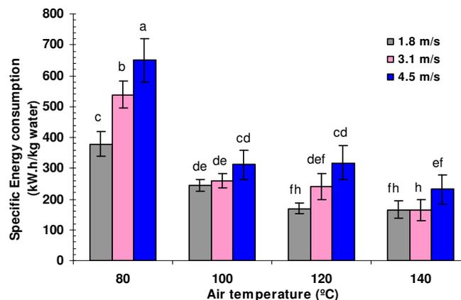
**Figure 10.** Specific energy consumption at different temperatures and drying air velocities.
