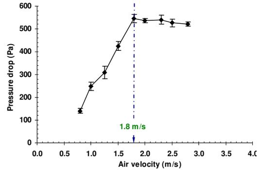
**Figure 1.** Fluidization characteristics of soybeans.
