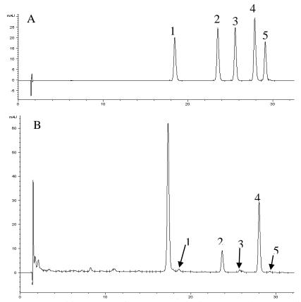
**Figure 2.** Chromatograms of flavonols and flavones: 1: Myricetin; 2: Quercetin; 3: Luteolin; 4: Kaempferol, 5: Apigenin and (A) Chromatogram of reference standards, (B) Chromatogram of Hongbaoshi sample of Sept. 3.
