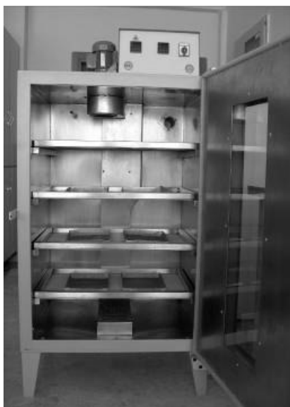
Figure 1. Laboratory type cabinet dryer used for oyster mushroom drying.
