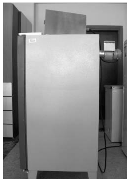
Figure 1. Laboratory type cabinet dryer used for oyster mushroom drying.
